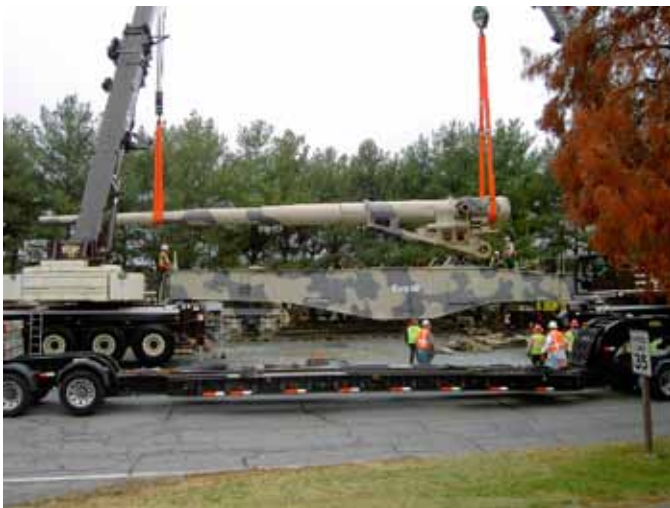
K5 barrel being lifted from gondola at APG
