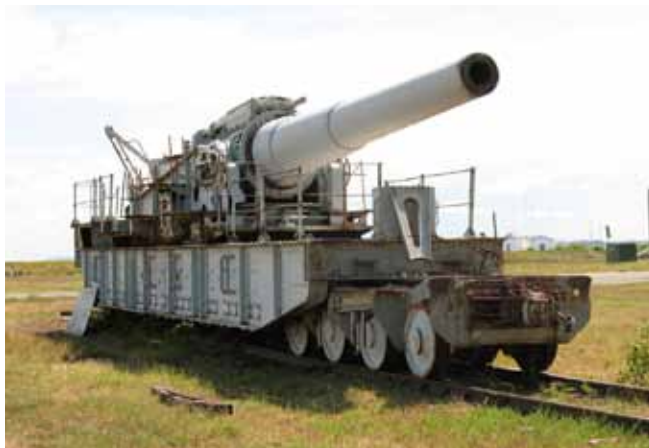
12-inch M1895 gun on its railway mount at Dahlgren
