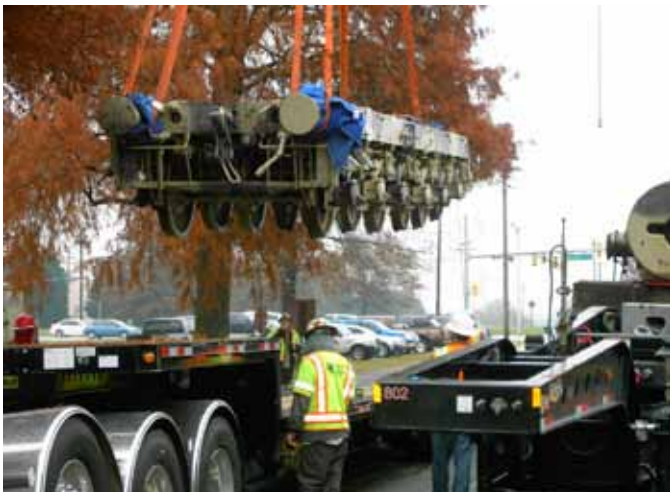
K5 rail truck being lifted at APG
