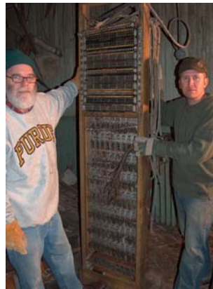
Leo Polaski and Andy Grant working on recovering one of the BD-74 Fire Control Switchboards from Fort H.G. Wright.
